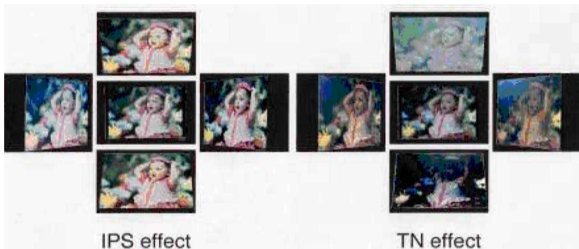
Figure 1. Display images of the IPS TFT-LCD and the TN TFT-LCD viewed from different directions.
